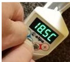
Press simultaneously the „NIGHT/ESC” and the „minus” buttons and hold them for approx. 9 sec
